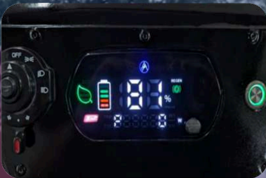
Smart Display For Charge % RPM, other Alert Signals
